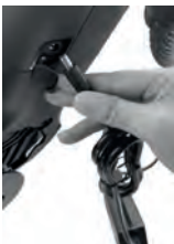
Battery charging on the bike
